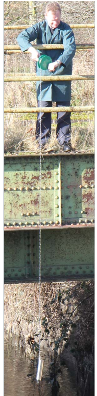
Liquid flows in when the sampler hits the bottom
