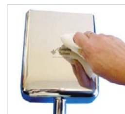
4. Clean etching area thoroughly using demineralised water
