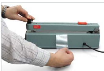
Cut the lay-flat tubing to length & seal one end
