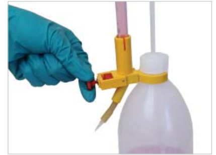
Screw in for accurate discharge
