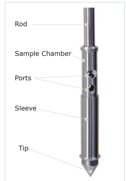
Different Volume Sampling Tips can be fitted to the same chamber
