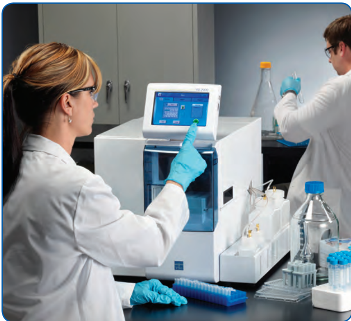
Figure 2 The YSI 2950 Biochemistry Analyzer can simultaneously measure up to six chemistries for raw materials, R&D, in-process and final product sample analysis.
