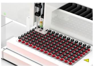
The fully automated samplers of the autoX series ensure an unmatched sample throughput in the vertical and horizontal operation mode. A special quartz container technology and the sophisticated protective covering of the sampler shield the charcoal from environmental impacts. An additional purging of the sample rack with inert gas is not necessary.
