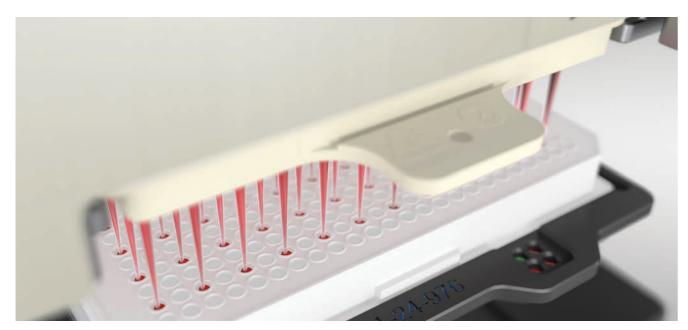
The first quadrant of a 384 well microplate is filled by a 96 channel CyBio SELMA using the microplate adapter 384.
