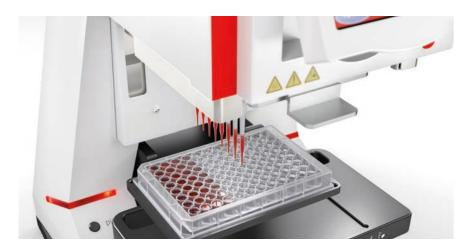
the microplate adapter 384. With this adapter, 384 well microplates can be processed quadrant-wise with the 96 channel CyBio SELMA\*1. The slide function makes handling very easy and shows you the currently processed quadrant ensuring precise and reliable filling of the 384 well microplates.
