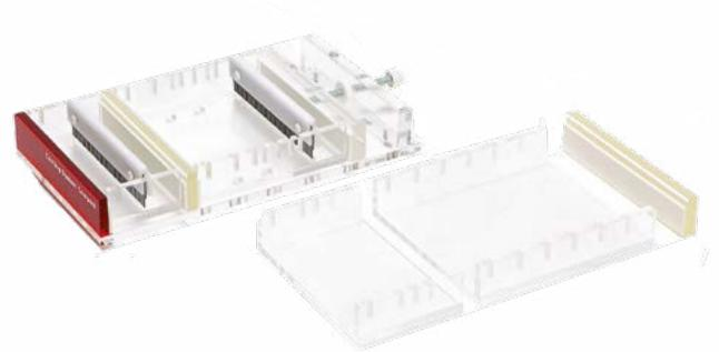
Casting System and optional casting dams for Compact Multi-Wide
